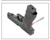
1. Push the fixing pin out sideways with a pin punch.
