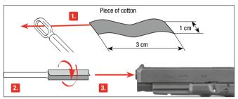
Prepare a thin rod with a length of approx. 30 cm. Attach a piece of cotton fabric to its end and clean the barrel with some silicone oil
